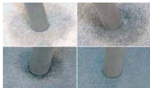
Oil traces on the surface after 144 h at room temperature
