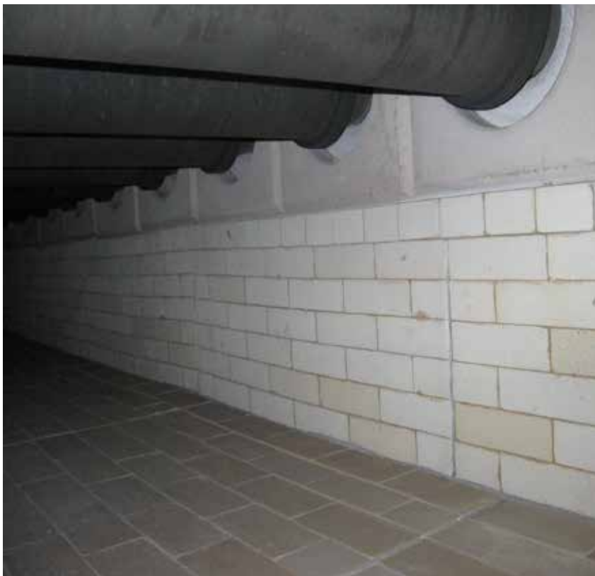
Roller hearth furnace 1050 °C with SILCAREF
