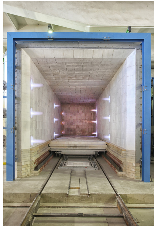
Bogie hearth furnace 1,350 °C with SILCASTACK combination modules
