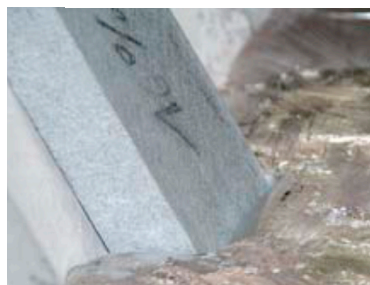
Wetting in liquid Aluminium
